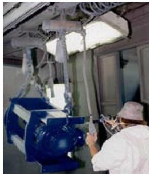
Fig. 5: Explosion-proof mechanical hoist
