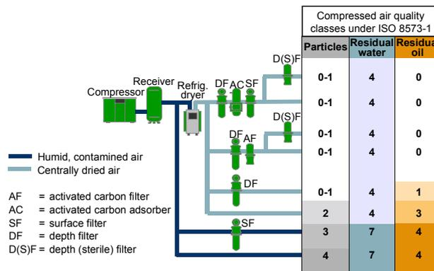
Fig. 12: Compressed air quality when using refrigeration dryers
