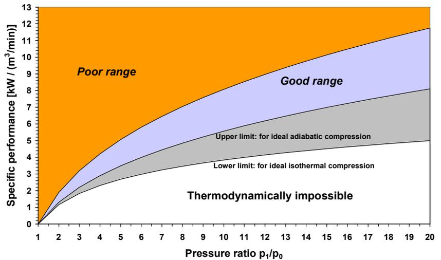
Fig. 4: Specific power demand for compressed air production
