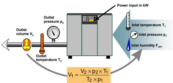
Fig. 1: Measuring the inlet volume flow rate
