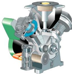
Fig. 3: Piston compressor
