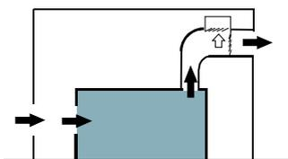
Fig. 10: Ducted discharge air in larger compressors
