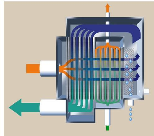
Fig. 3: Heat exchanger with integrated condensate trap (demister)
