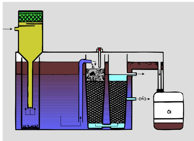
Fig. 11: Static oil/water separation system
