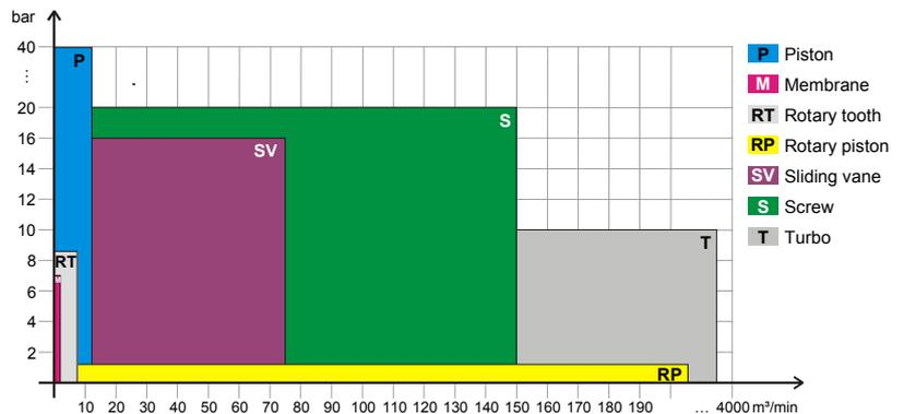
Fig. 2: Potential power of compressor types
