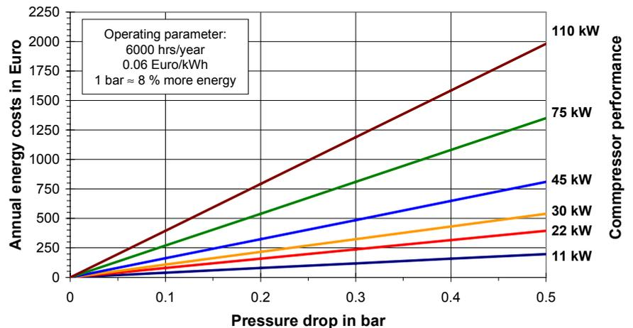
Fig. 6: Energy costs due to pressure drops
