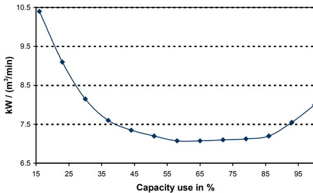
Fig. 5: Specific performance of a speed-controlled compressor
