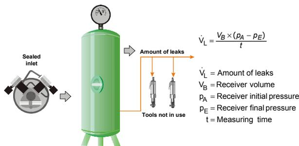
Fig. 9: Measuring leaks by draining compressed air receiver
