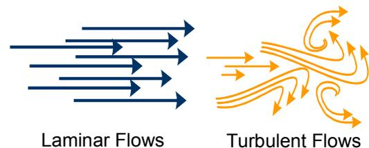
Fig. 5: Laminar and turbulent flows
