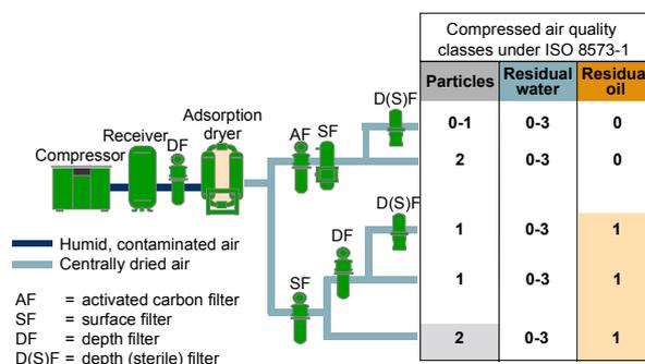
Fig. 13: Compressed air quality when using adsorption dryers
