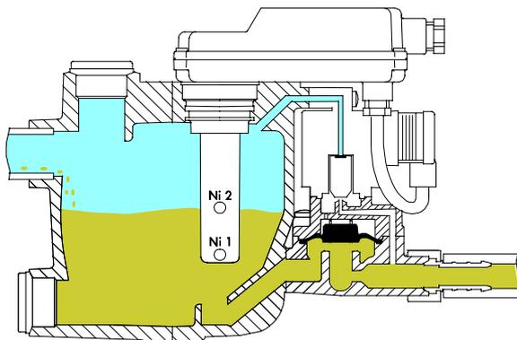
Fig. 10: Level-controlled separator
