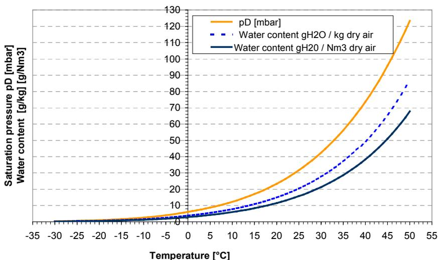
Fig. 3: Saturation pressure and water content of air
