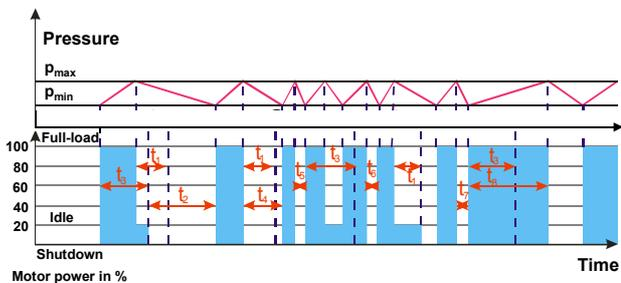
Fig. 3: Range of application base load compressor
