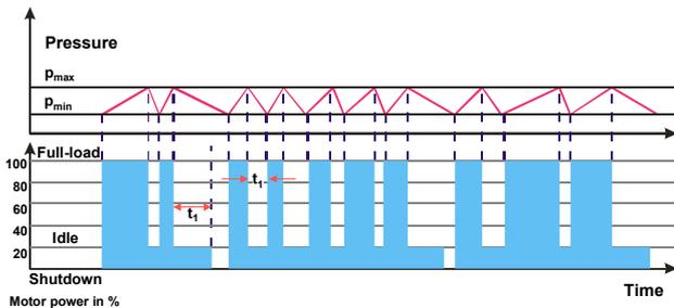
Fig. 2: Range of application peak load compressor
